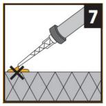
6. IMPORTANT Do not entrap air into the hole. Inject the Product into the perforated sleeve starting from the bottom, while slowly drawing back the static mixer
